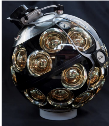
Figure 1: Side view of a KM3NeT DOM.
